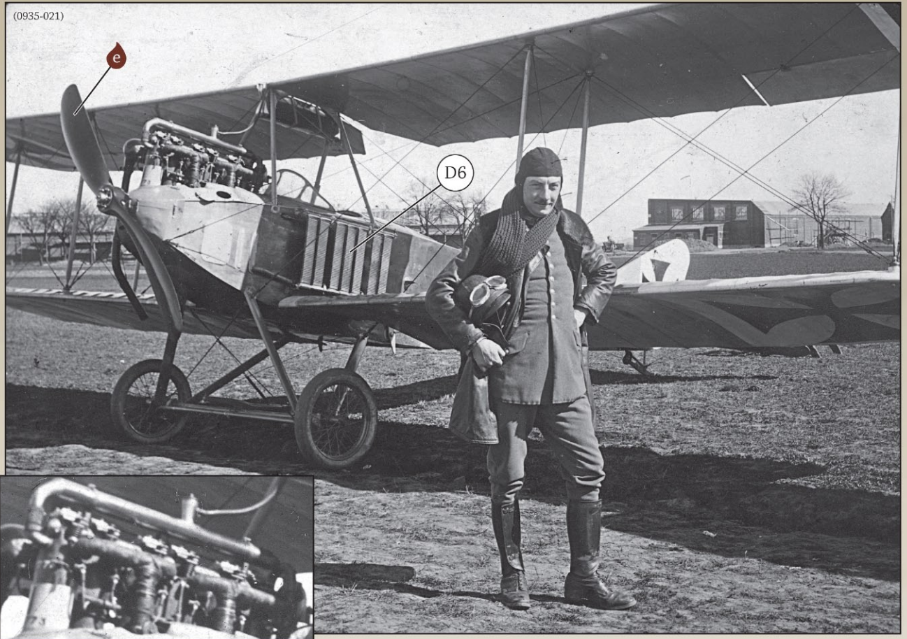
This unidentified Albatros B.II is powered by a 100hp Daimler-Mercedes D.1 engine and features uncovered wire wheels, a thin version of the 'elephant' exhaust and a darkly painted propeller. Note the opaque wing fabric precluding a CDL finish. The airman is noted as being 'Unteroff Breidr' and is not wearing any identifiable pilot or observer badges.
