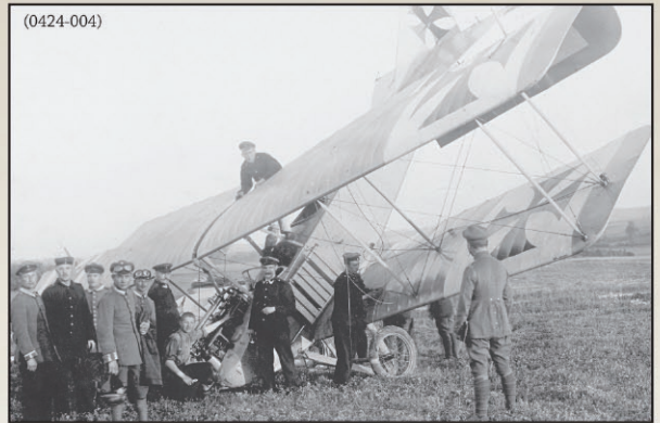
The occupants of this unidentified Albatros built B.II appear to have escaped serious injury following a rough landing. Note the overall dark, opaque, nature of the fabric surfaces, uncovered wire wheels and 120hp Daimler-Mercedes D.II engine.
