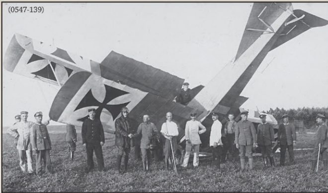
The occupants of this unidentified Albatros built B.II appear to have escaped serious injury following a rough landing. Note the overall dark, opaque, nature of the fabric surfaces, uncovered wire wheels and 120hp Daimler-Mercedes D.II engine.
