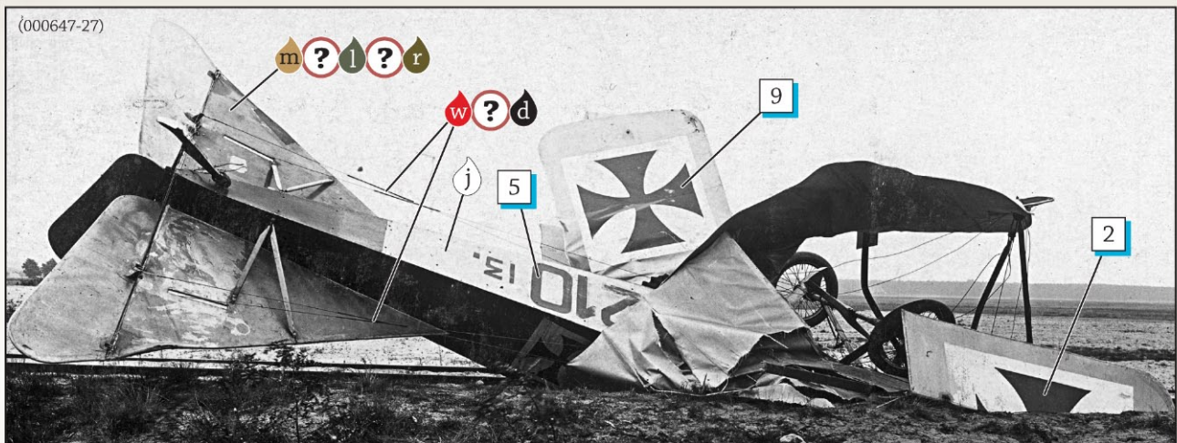
(000647-27) The heavily weathered and patched tailplane is obvious in this photo. A large portion of the bottom of the fuselage appears to have been painted white so that the oversize serial number was more visible from the ground, indicating that Albatros B.II 210/13 was probably being used for training at the time of this crash. Note the dark material w ? wrapped around the elevator control cables where they cross 'over' each other.
