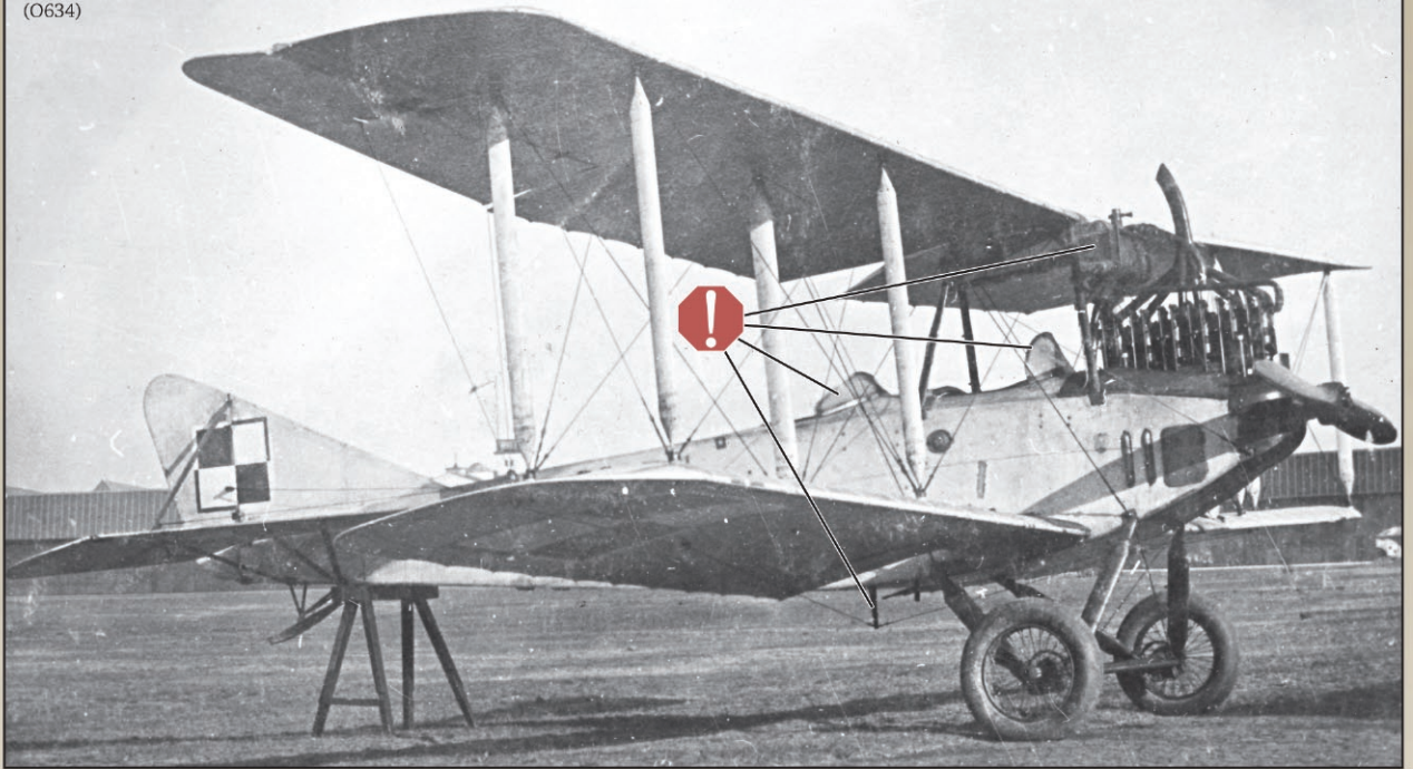
Roland built 110hp Benz Bz.II powered Albatros B.IIa in Polish service with stick type control column, radiator in front of the top wings and large balloon type tyres. The thick wooden interplane & undercarriage struts are an identifying feature of later production B.IIa. Note the Albatros C.1 style tail skid and tailplane bracing frequently found on late production B.II or retrofitted to older aircraft.
