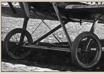
< Undercarriage detail from the unidentified Albatros B.II seen on page 23. Note the claw brake spring wired to the undercarriage bracing cables and the uncovered wire wheels. The suspension bungee cords are protected by leather bags.
