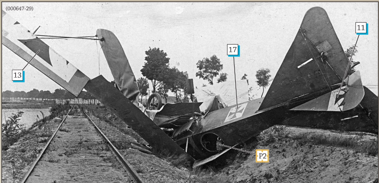
(000647-29) Albatros B.II 210/13 has crashed into a ditch beside some railway tracks. Note the pilot's safety belt hanging from the rear cockpit opening and the mismatched, heavily patched, tailplane components.
