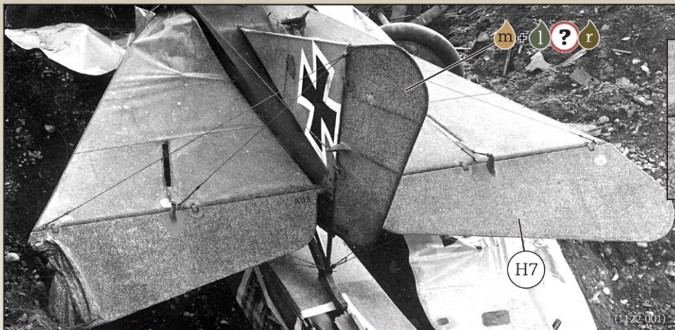
Tailplane detail from an unidentified crashed Albatros B.II showing factory applied 'sponge rolled' camouflage finish on the upper surfaces.
